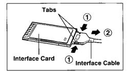
While pressing the side tabs of it ( $\bigcirc$ ), pull the interface cable straight ( $\bigcirc$ ).
